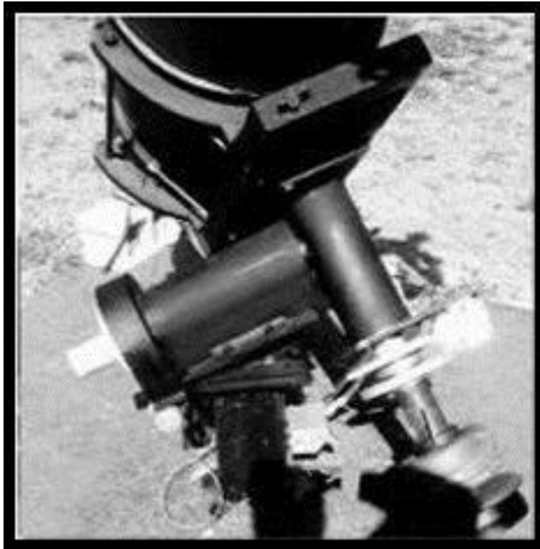
Figure 4. Telescope pier and wedge is made from two, 1/2-inch 9" x 12" steel plates welded together.
