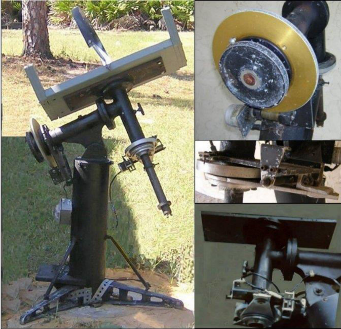
Figure 6. LEFT: Parks German equatorial mount with UPPER RIGHT Thomas Mathis 10-inch worm gear drive using a 1/2-RPM Hurst motor [Transmission ratio: (25/57) (1/315) = 0.5 / 718.2 = 1 / 1436.4 ]. CENTER RIGHT: A 14-inch tangent arm declination drive with DC motor and a machined clutch assembly. The drive gear is a 6-inch, 1/2"O.D. brass gear and threaded aluminum block was machined for smooth and precise fit. BOTTOM RIGHT: Another view of equatorial head and Dec drive. (Note spider webs, other bug debris and corrosion from years of use).
