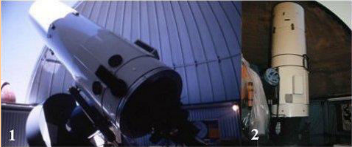
Photo-1: 24-inch f/75 Boller and Chivens Cassegrain telescope (UH24). Photo-2: Another view of UH24. This telescope and dome are gone and replaced by huge 8-meter telescope.
