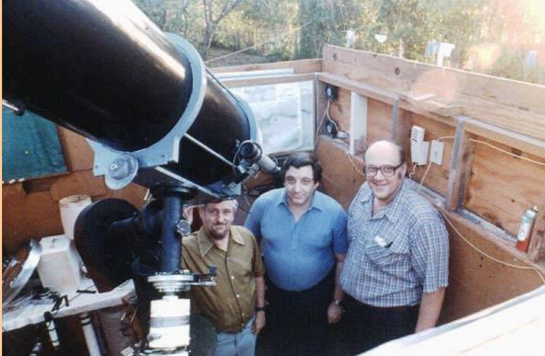
Chick Capen, me and Don Parker in my Cutler Ridge, Florida (1980) observatory under my homemade 12.5" f/30 Cassegrain
