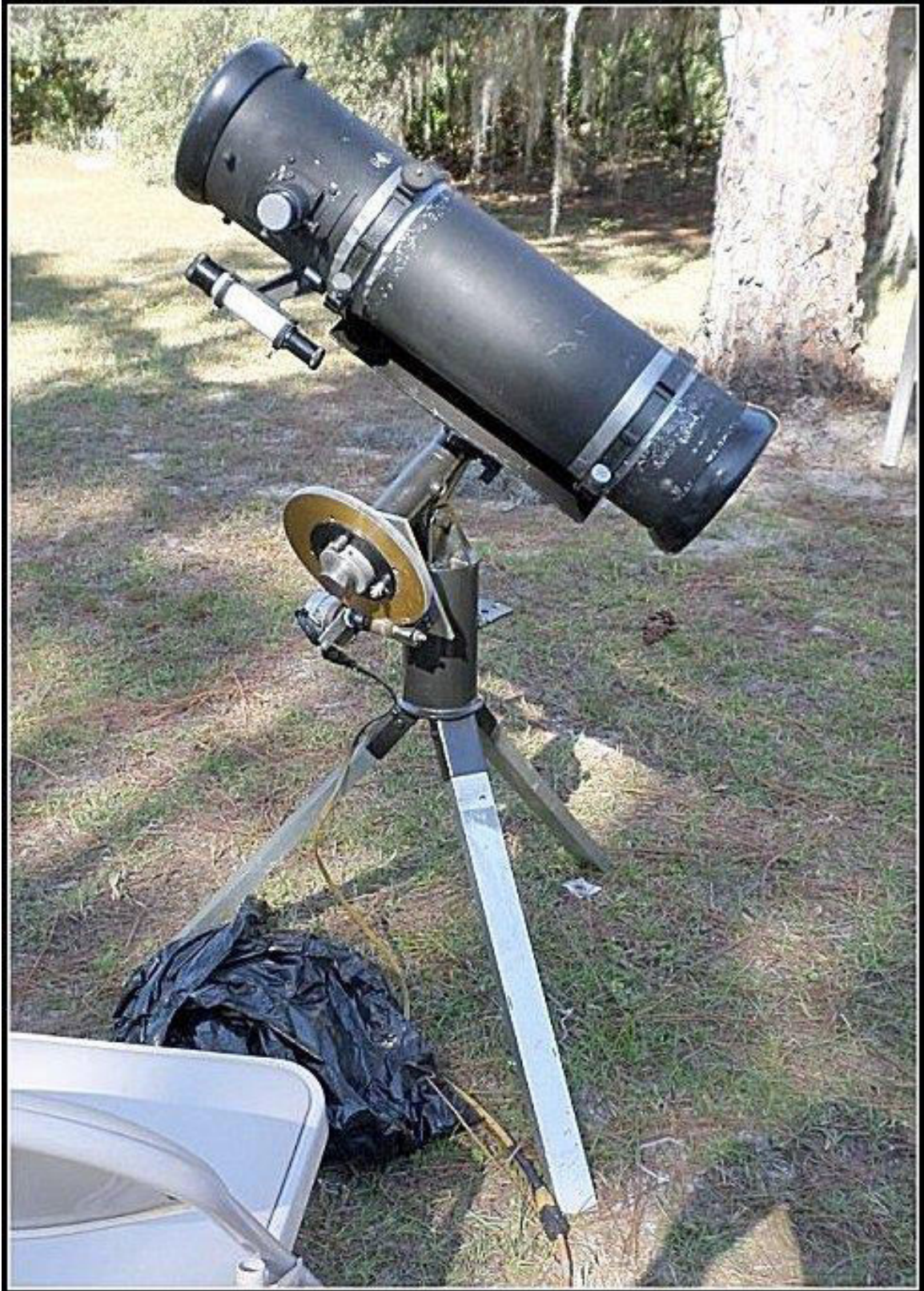
6" f/4 Newtonian telescope attached to restored mount using Orion tube rings.
