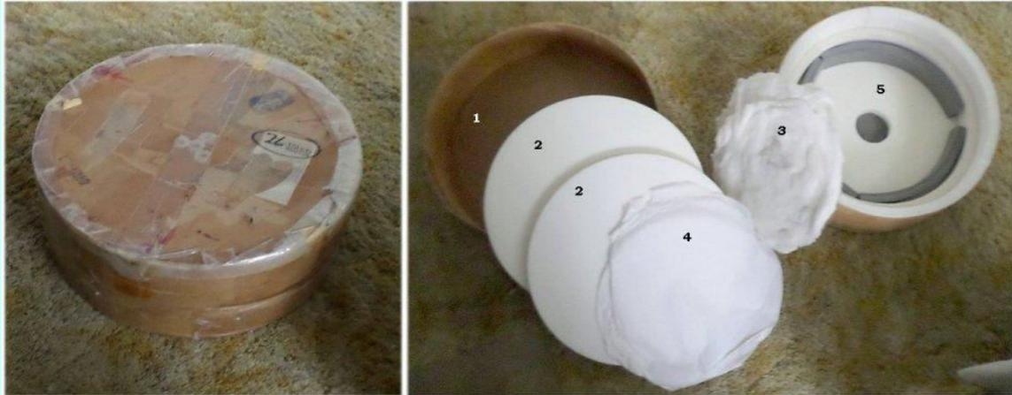
Figure 6. LEFT: 16" magnetic tape shipping container. RIGHT: 1) container top, 2) two thin sheets of Styrofoam (with a place for secondary mirror and holder, 3) Sheet of cotton glued to 1/8 th-thick Plexiglas disk, 4) tissue paper and 5) bottom of container with Styrofoam bottom, side sheets and three soft rubber forms (gray).
