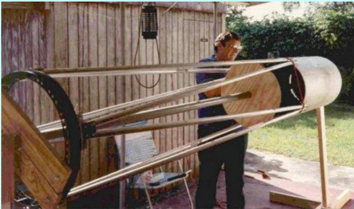
Figure 2a. Photograph of 16-inch f/6.9 Newtonian Reflecting Telescope simple truss tube assembly being constructed on author's patio. A chain link fence post to be fitted into two plywood circles and components were then assembled in turn to complete telescope. Open tube truss system design reduces weight by 50%.
