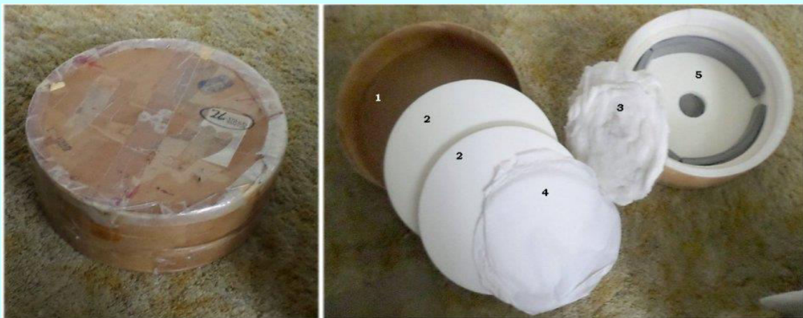
LEFT: 16" magnetic tape shipping container. RIGHT: 1) container top, 2) two thin sheets of Styrofoam (with a place for secondary mirror and holder, 3) Sheet of cotton glued to 1/8th-thick Plexiglas disk, 4) tissue paper and 5) bottom of container with Styrofoam bottom, side sheets and three soft rubber forms (gray).
