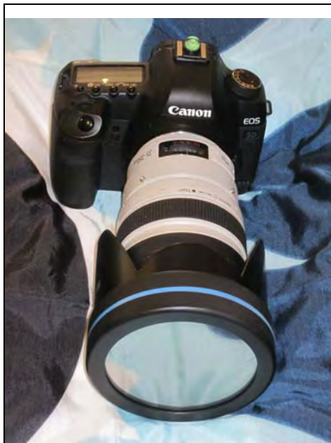
Figure 5. A front-mounted glass solar filter for imaging the partial solar eclipse phases. Credit: Dr. Mike Reynolds.
