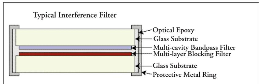
quarterwave thick. This sandwich of quarterwave layers is made up of an alternating pattern of high and low index material, usually zinc sulfide and cryolite, respectively. Together, the quarterwave coatings forming the reflective layer is called a stack. The combination of two stacks and the spacer comprise a one cavity bandpass filter. The number of layers in the stack is adjusted to tailor the width of the bandpass.
