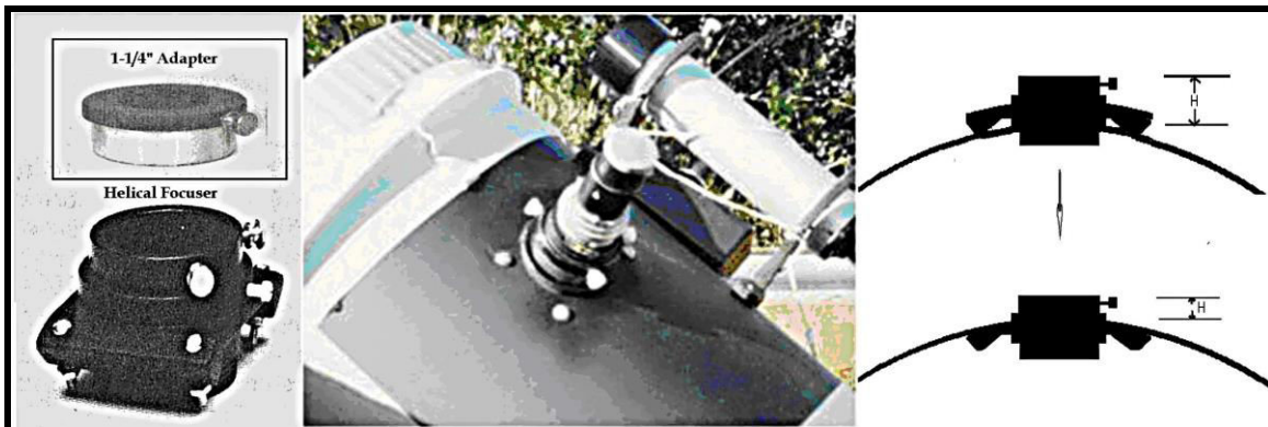
Figure 2. LEFT: Novak low profile helical focuser with 1-1/4-inch adapter insert. CENTER: Low Profile focuser with fine helical adjust with built-in Barlow lens. RIGHT: Helical focuser mounted from inside of tube and saves 1/2-inch of distance from secondary mirror to focal plane.
